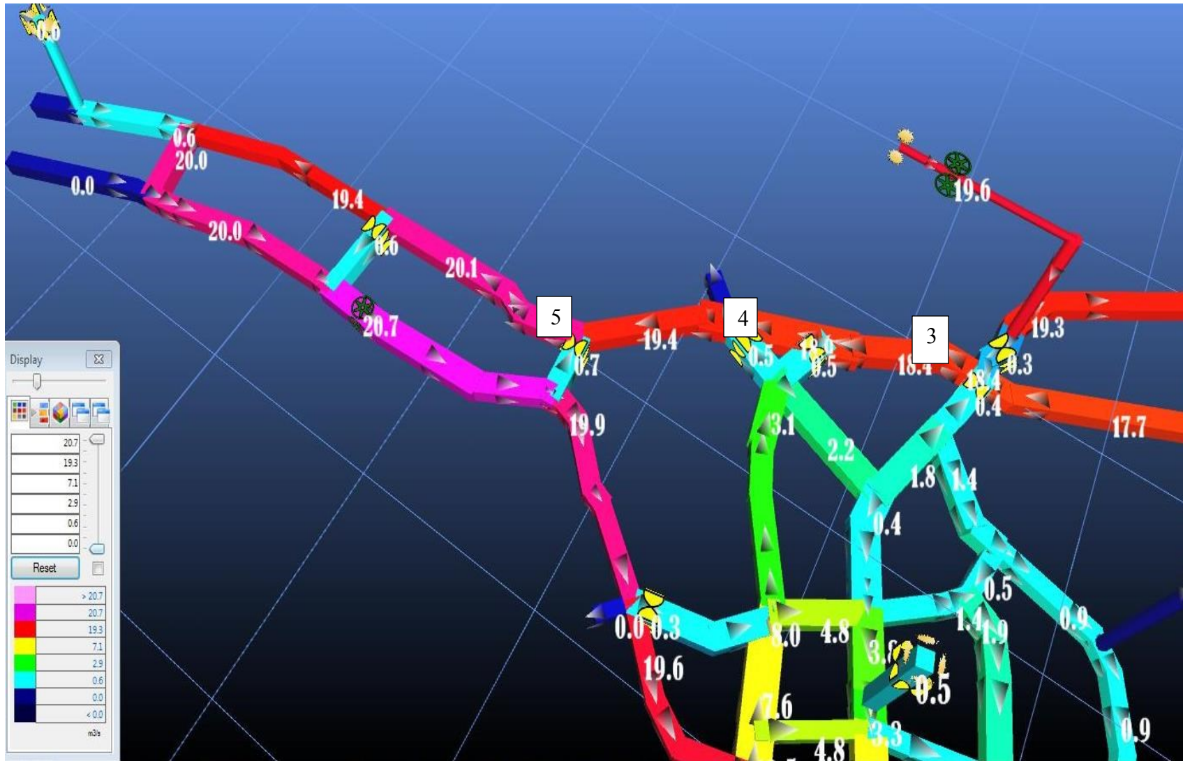
Figure 5.13 Main fan and west booster fan at blade set 5 simulated results
